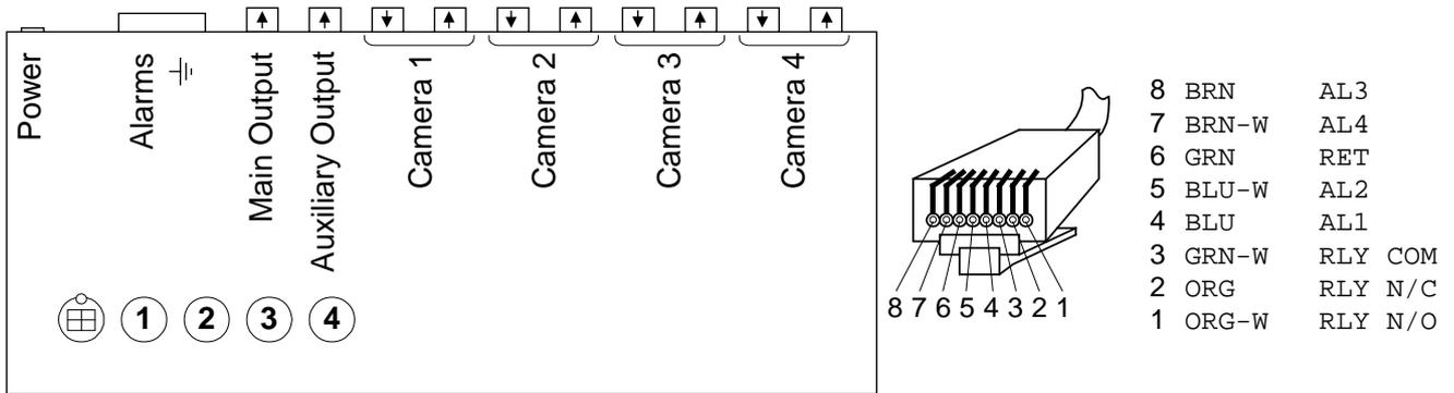
Connect your alarm contacts (floating, voltage free) to AL1-AL4 and connect their commoned returns to RET. See section *Specifications* for alarm relay contact details.
