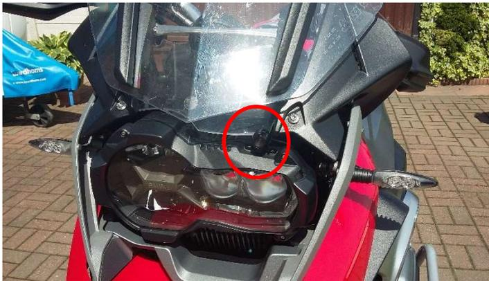
The camera wires were simply routed through the frame and secured with tie wraps. Some panels were taken off to make this task easier. There's an excellent video on Youtube on how to remove the panels on a BMW GS titled "R1200GSw Bodywork and Tank Removal and Installation 2013+" by jimvonbaden1.
