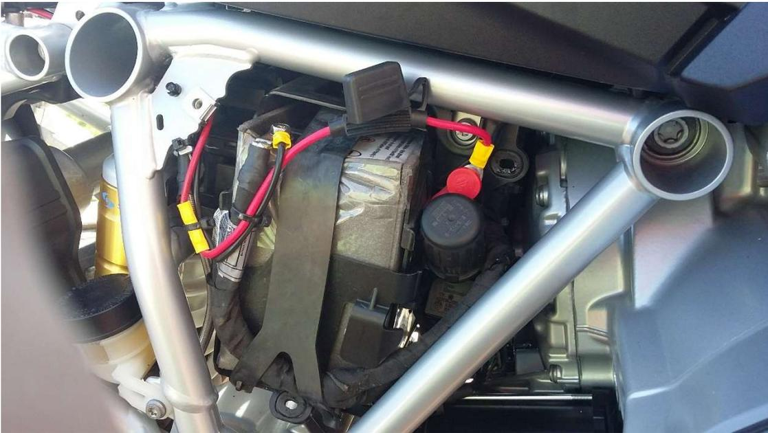
We then routed a pair of power wires through the frame up to the pillion seat where the DVR was located.
