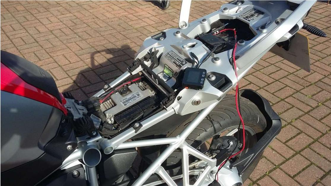
In this installation we used a **“Smart Power Supply”**. The Smart power supply works by switching on the DVR when vibration is detected, so this was securely strapped to the bike module under the seat. Using the smart power supply means we can take a power feed straight from the battery and doesn't require an ignition circuit, which can be difficult on a CAN bus based bike.
