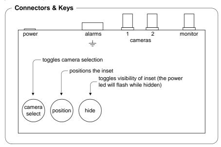
A supplementary earth (screw) connection is provided, it's located beneath the alarm connector.
