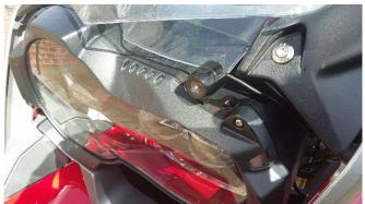
The camera wires were simply routed through the frame and secured with tie wraps. Some panels were taken off to make this task easier. Theres an excellent video on Youtube on how to remove the panels on a BMW GS titled "R1200GSw Bodywork and Tank Removal and Installation 2013+" by jimvonbaden1.
