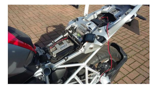
In this installation we used a **"Smart Power Supply"**. The Smart power supply works by switching on the DVR when vibration is detected, so this was securely strapped to the bike module under the seat. Using the smart power supply means we can take a power feed straight from the battery and doesn't require an ignition circuit, which can be difficult on a CAN bus based bike.
