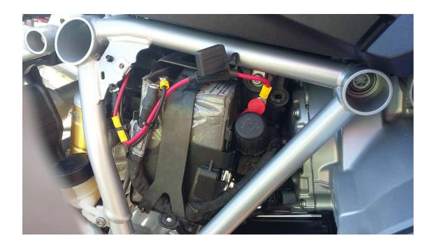
We then routed a pair of power wires through the frame up to the pillion seat where the DVR was located.
